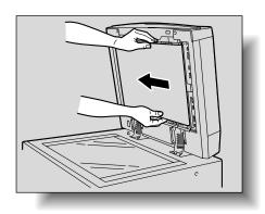
3 Clean the newly exposed surface of the belt by wiping it with a soft cloth dampened with a mild household detergent (as in step 1).
